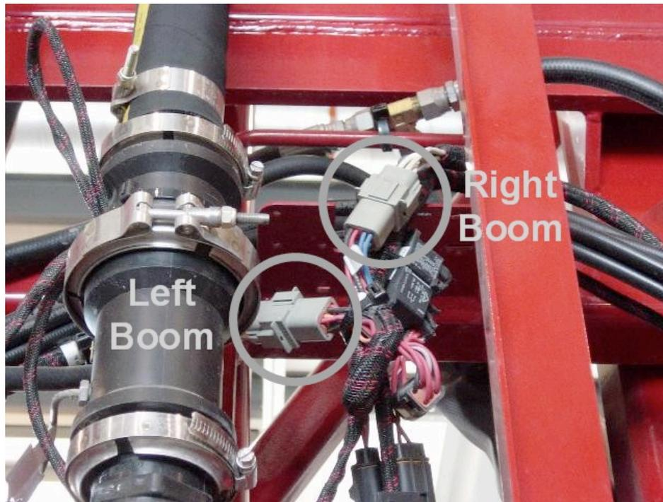
2. Disconnect the plugs from the left boom and plug the SprayTest "Left Boom" plugs into them.
